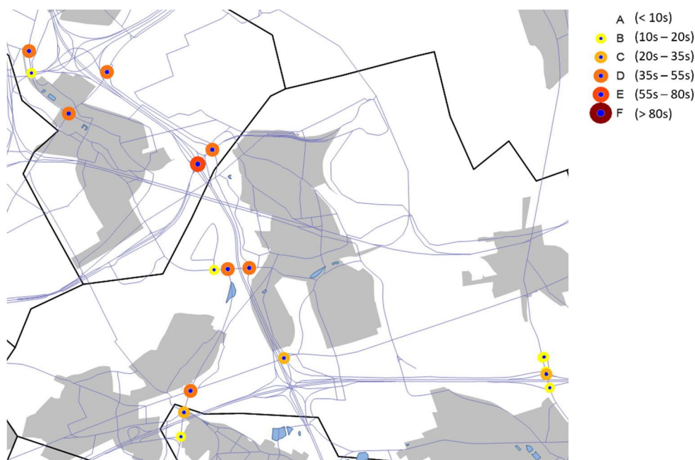
Figure 55 : Analyse LOS alternative G3A1, zone Zaventem - HPM
